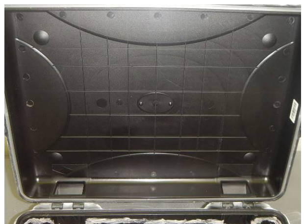
Picture 6 Sinora Case SIN-05542-20BK without visible dust inside after the solid foreign objects test IP6X
