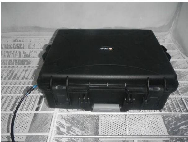
Picture 3 Sinora Case SIN-05542-20BK in the dust chamber 89 with under pressure hose before the solid foreign objects test IP6X
