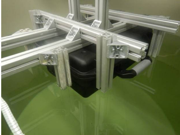
Picture 7 Sinora Case SIN-05542-20BK mounted in immersion frame during the immersion test IPX7
