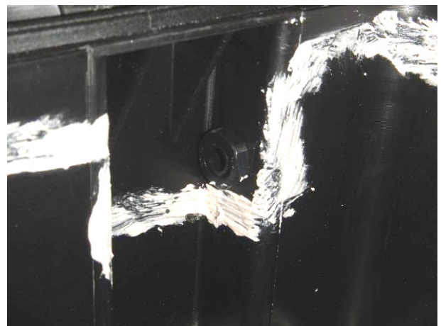
Picture 10 Sinora Case SIN-05542-20BK without visible water inside during the immersion test IPX7
