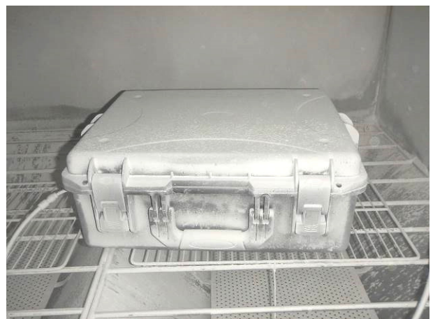
Picture 4 Sinora Case SIN-05542-20BK with settled talcum dust after the solid foreign objects test IP6X
