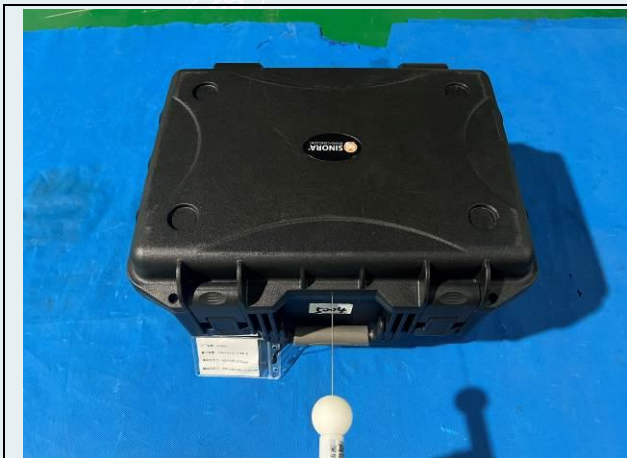
Fig.1-5 Metal probe inspection before test
